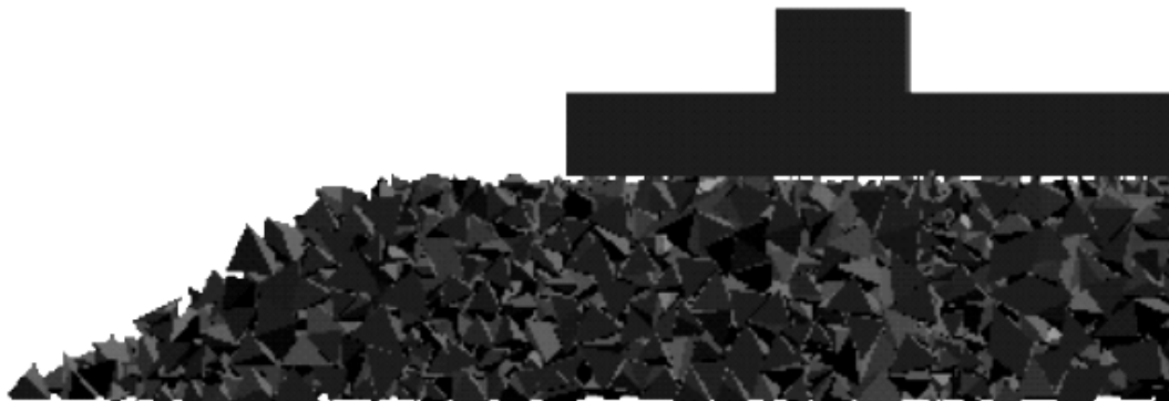
Figure 3. Ballast Sample of a Half Railroad Section with Angular and Cubical Aggregates of Shape Library 1
