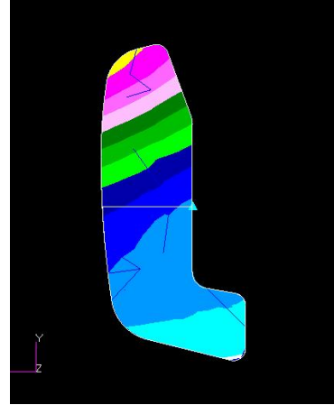
FIGURE 5.c: 2.5 Inch Debonded Area
