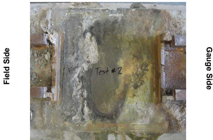
Figure 8: Worn rail seat surface treatment on the field side after 3 million cycles
