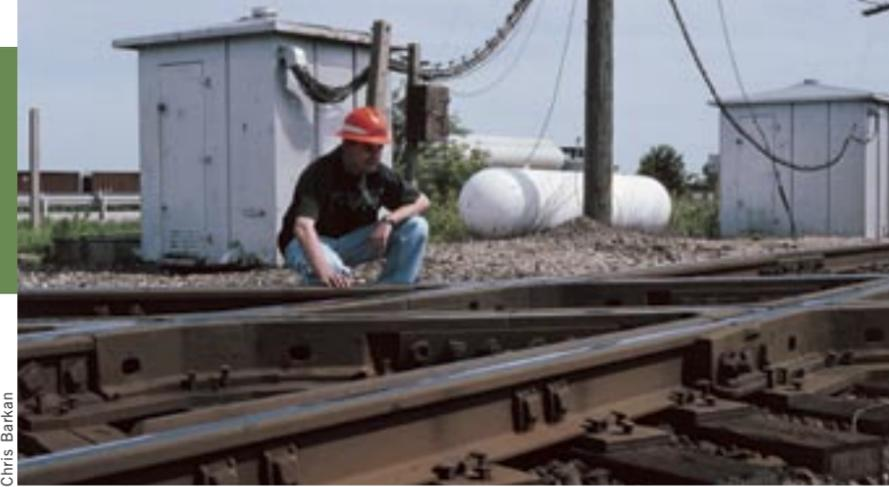
University of Illinois student Tyler Dick inspects the Union Pacific/Norfolk Southern diamond at Dwight, Ill., for damage due to high-impact loads in June 2000.
