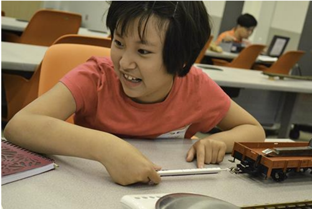
During the Rolling Resistance Measurement activity, a student takes a measurement on a railcar equipped with rubber tires.
