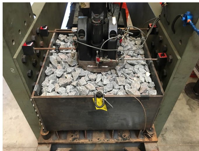
Figure 3. UIUC designed ballast box and loading plate
