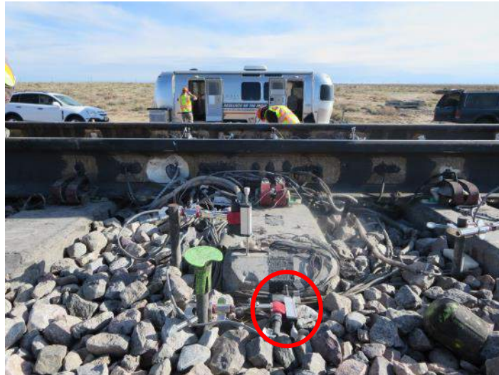
Figure 140. Lateral Crosstie Displacement Measuring Potentiometers
