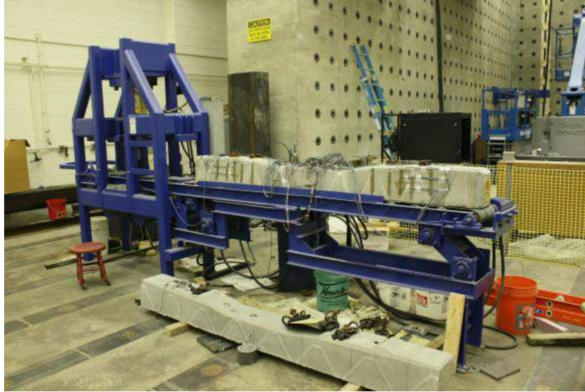
Figure 225. STT at UIUC Used in the Laboratory Experiment and FE Model Validation
