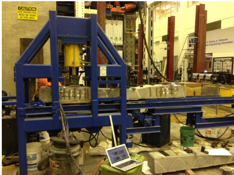
Figure 60. Vertical Rail Seat Loading Applied Using the STT
