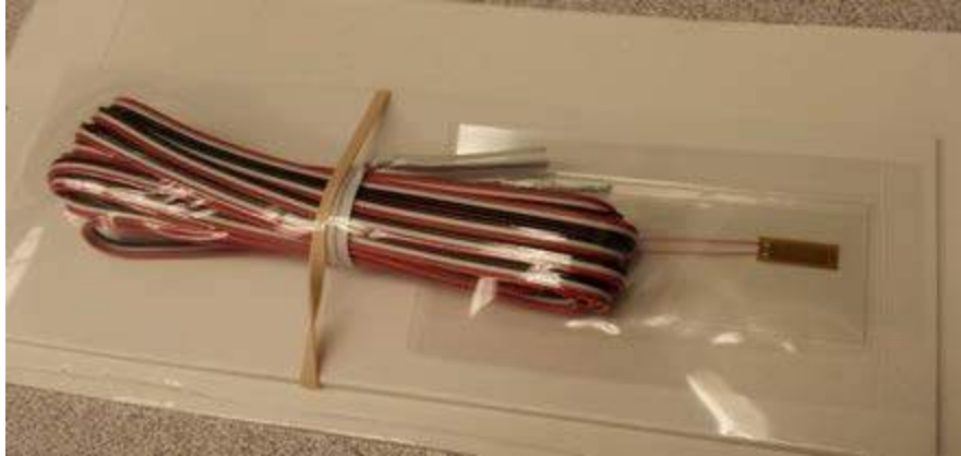
Figure 15. Standard 120-ohm Foil Type Shear Strain Gauge
