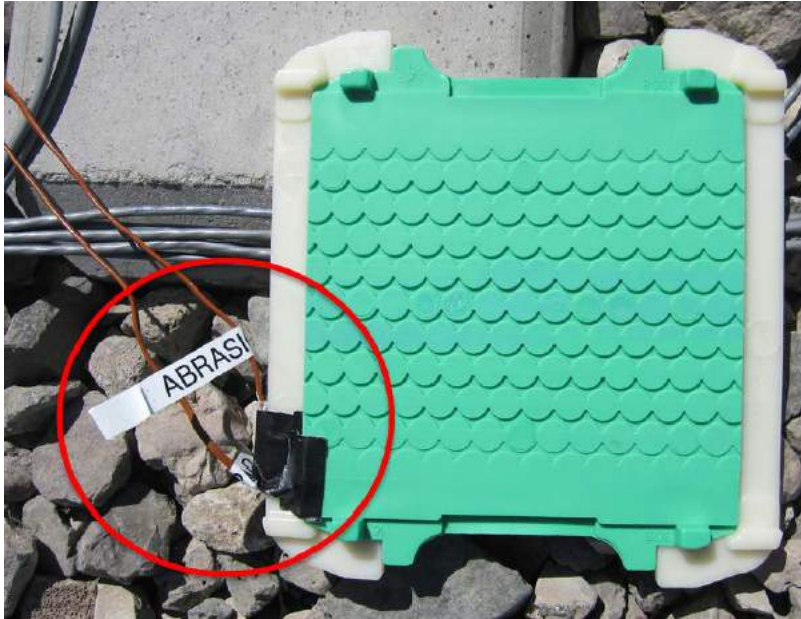
Figure 133. Instrumented Rail Pad with Thermocouple Wires on the Side
