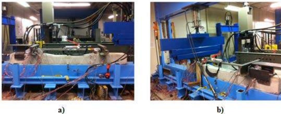
Figure 47. a) Lateral Force Applied by PTLF b) Lateral and Vertical Forces Applied by PTLF and SLTM Loading Head
