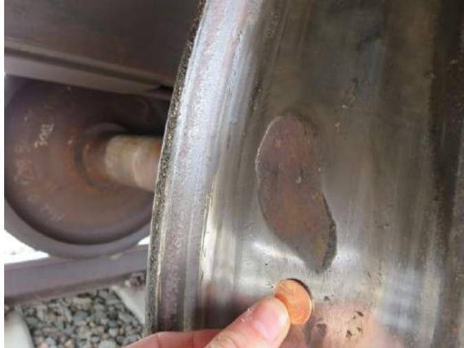
Figure 147. Large Flat Spot on the Wheel of Freight Consist
