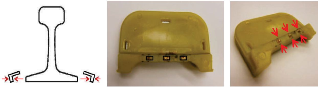
Figure 130. Insulator Post Compression; Location of Strain Gauges; Direction of Strain (left to right)
