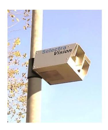
Video camera and 3D laser scanner are integrated in the same box
