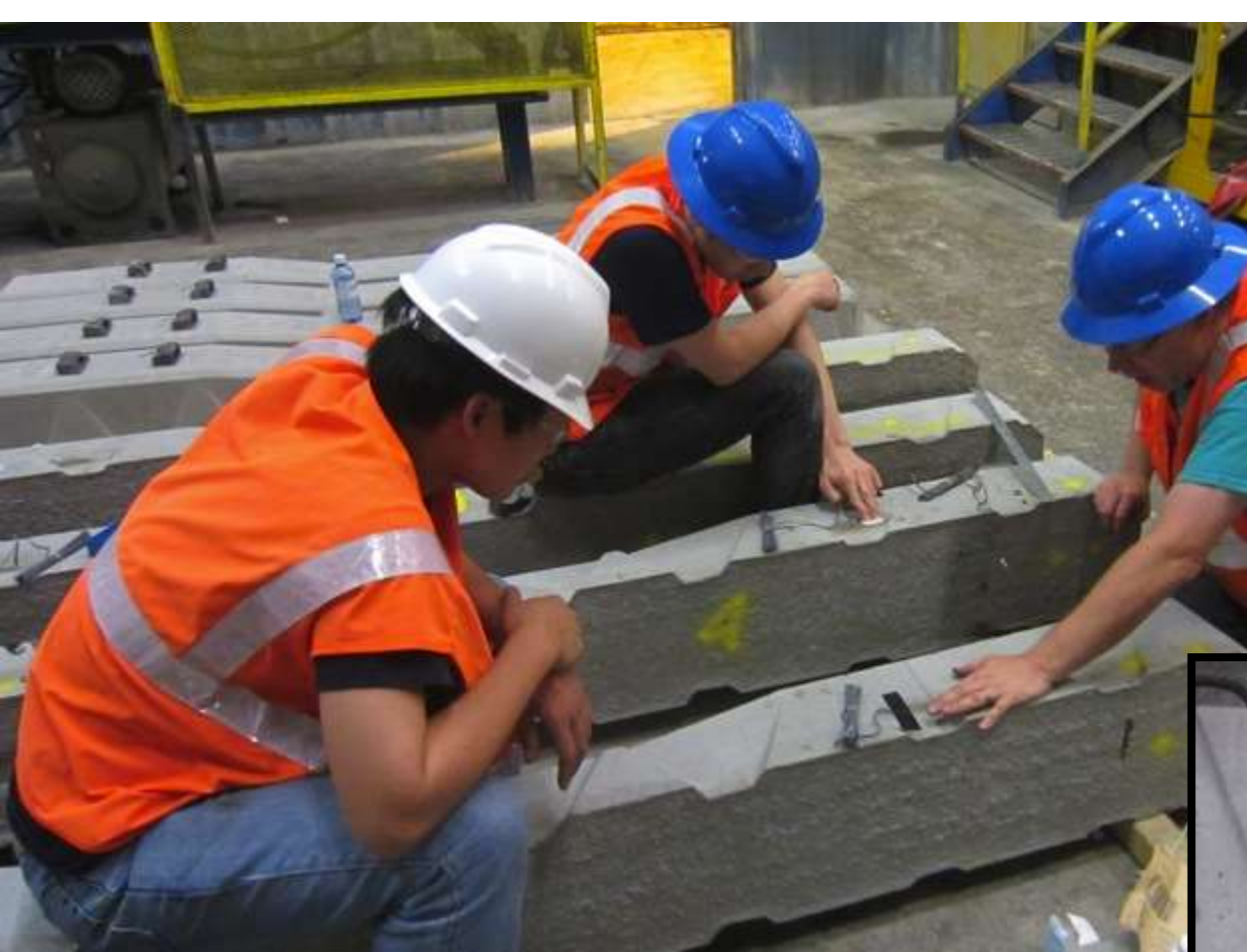
Placement and protection of surface strain gauges
