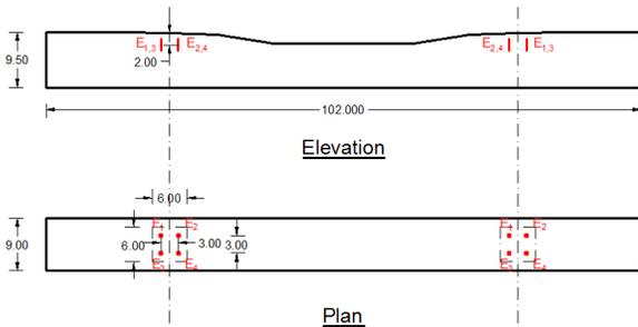
**FIGURE 3 LOCATIONS OF CONCRETE EMBEDMENT STRAIN GAUGES BELOW RAIL SEATS**
