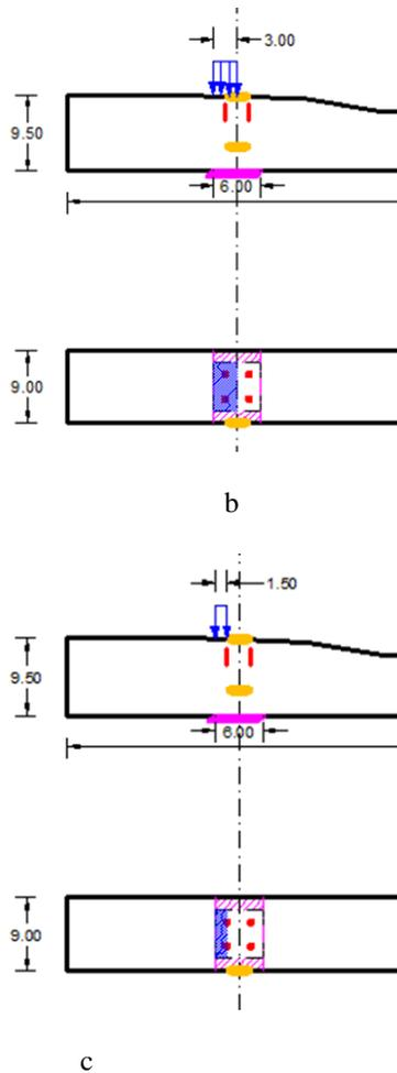
**FIGURE 5 LOADING AND SUPPORT CONDITIONS FOR RAIL SEAT COMPRESSIVE TEST**
