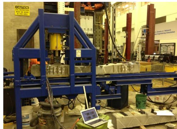
**FIGURE 1 STATIC TIE TESTER (STT)**
