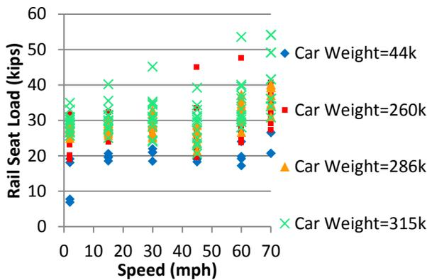
**FIGURE 11 RAIL SEAT LOADS AT RAIL SEAT U**
