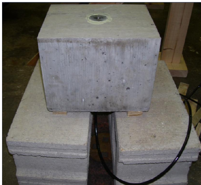
Figure 6.2 Concrete block prepared with pressure transducer
