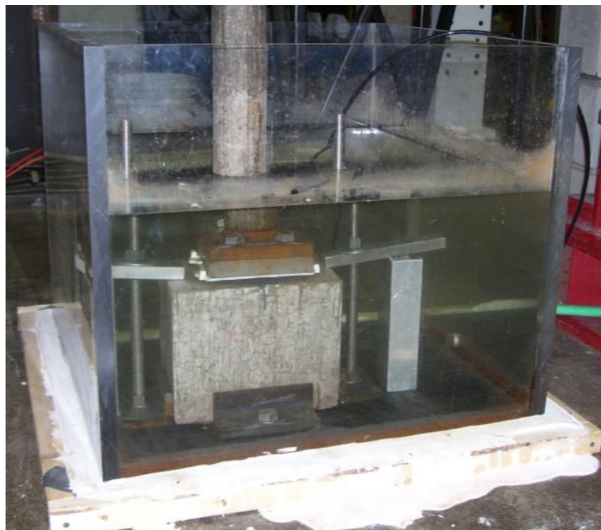
Figure 6.4 Close-up of the water tank of the mechanically-driven test apparatus
