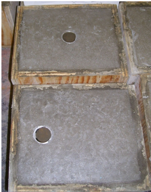
Figure D.4 Bottoms of the rail seat blocks during the first 24 hours of curing
