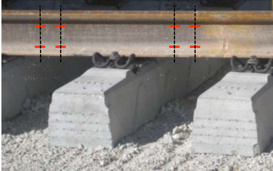
Lateral built-up load cell
