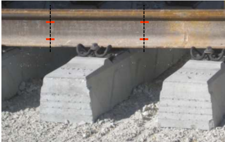
Lateral built-up load cell
