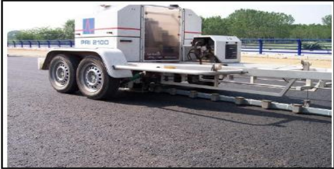
Falling Weight Deflectometer for assessing Structural Competency
