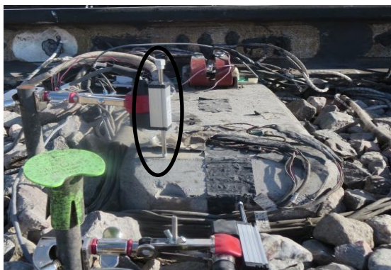
Figure 4 : Vertical crosstie displacement
