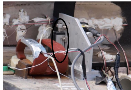
Figure 3 : Vertical rail displacement fixture
