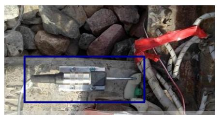
Potentiometer measuring pad lateral displacement
