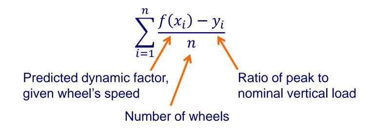
Additional "signed difference" metrics were developed, with weight given each for vehicle speed and nominal wheel load
