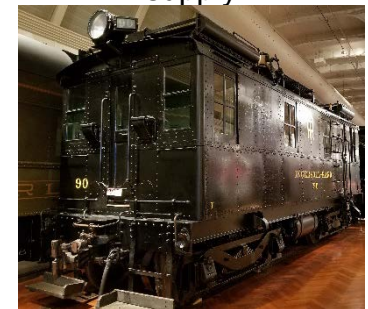
First commercially successful diesel-electric locomotive 1924, built by GE, Ingersoll-Rand, & Alco
