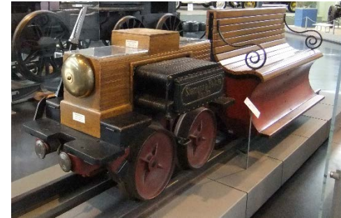
Replica of Siemens Electric Railway 1879, 3 rd rail supply
