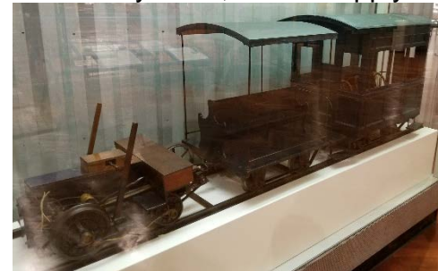
Model of Edison (GE) Electric Railway 1880, running rail supply
