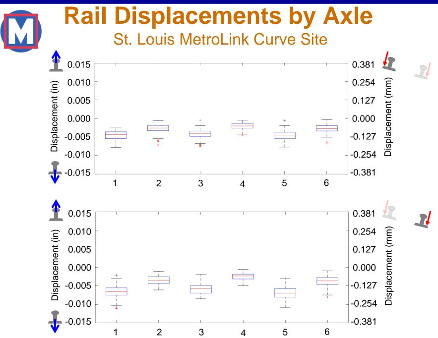
Quantification of Rail Displacement under Light Rail Transit Field Loading Conditions
