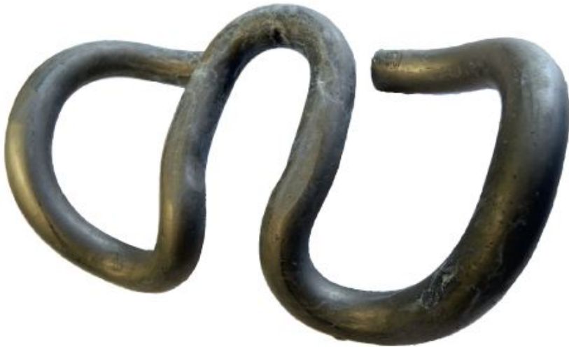
Photo 3: NiroTec® coating after 480 h
