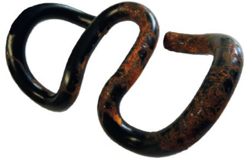
Photo 4: KTL coating after 480h
