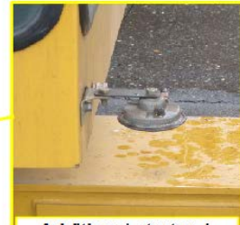
Additional startup / proximity alarms on cab
