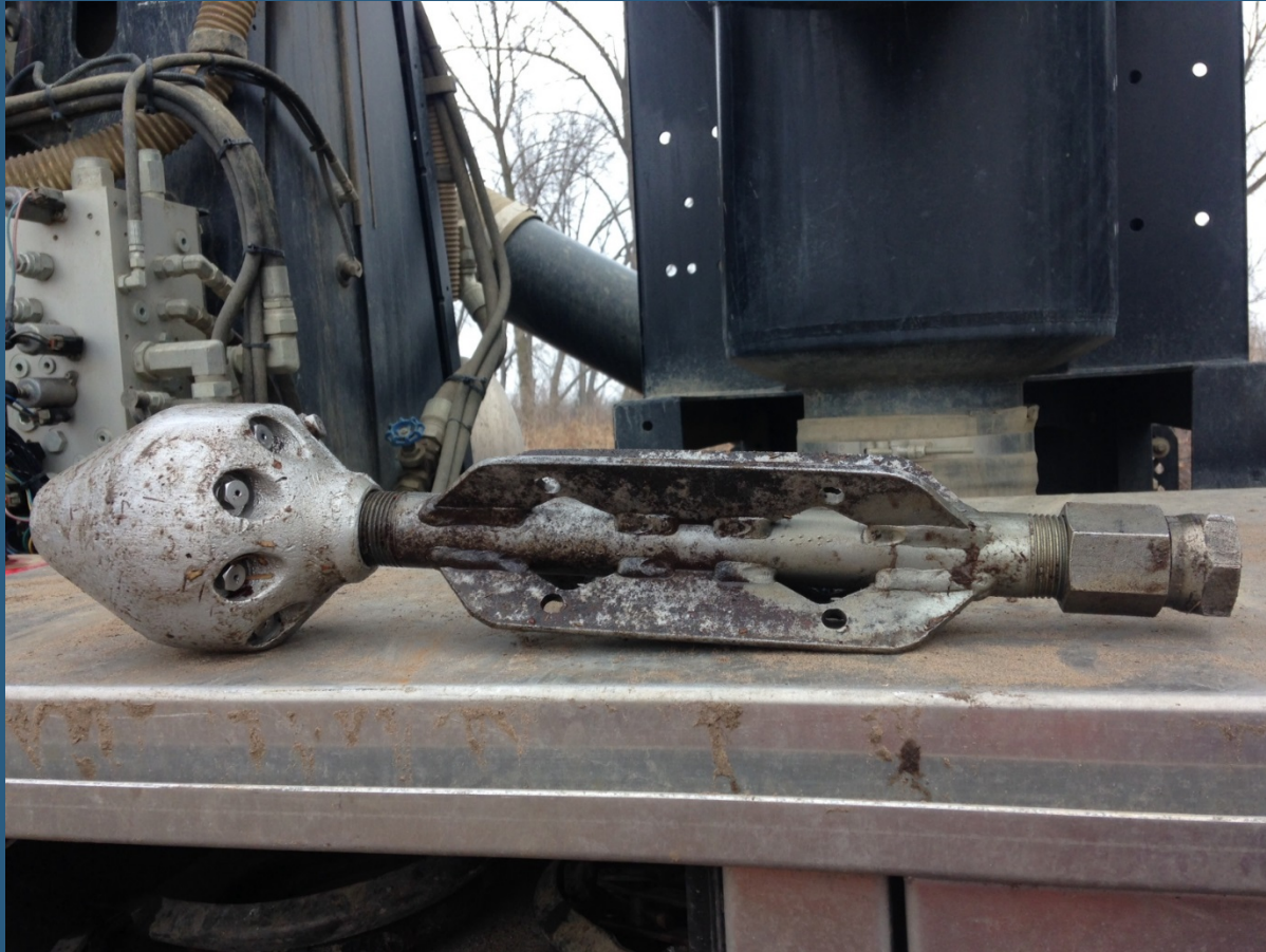
Nozzle head for high-pressure water jet cleaning brick sewer
