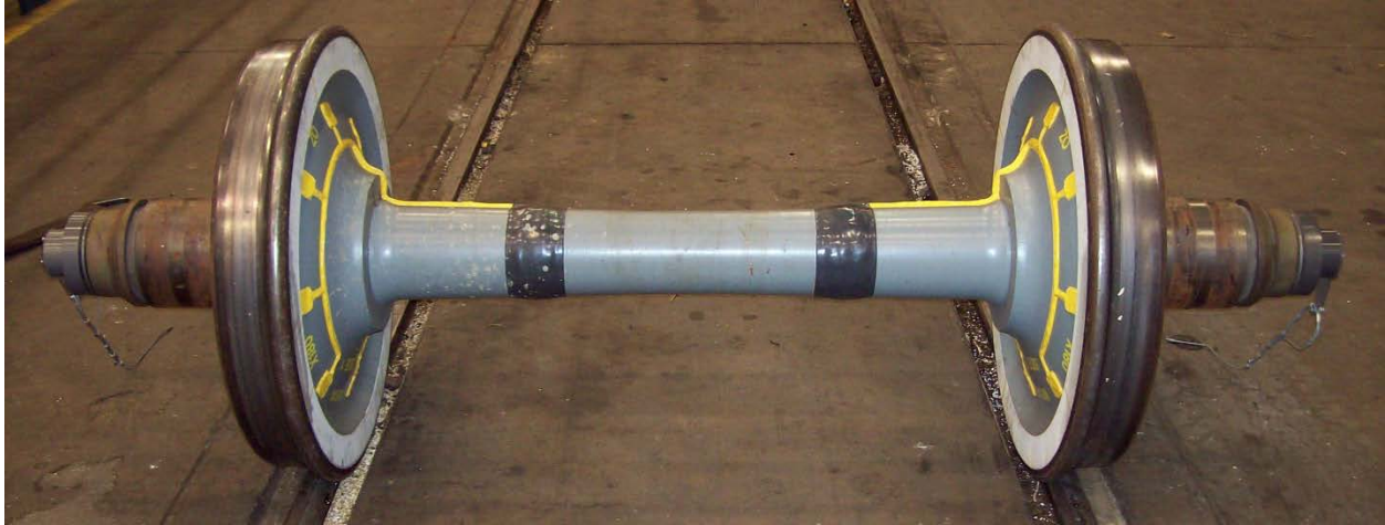
Figure 4.1 An instrumented wheel set used for research and development (TTX Company)
