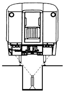
Figure 1: Camera Perspective From Beneath Railcar
