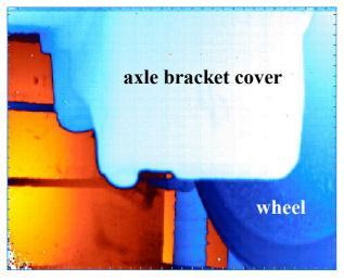
Figure 4: Infrared Image of Locomotive Wheel
