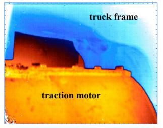
Figure 6: Infrared Image of Traction Motor Edge
