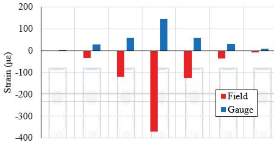
Figure 9: Strains in high rail from 40kips vertical and 20kips lateral load.
