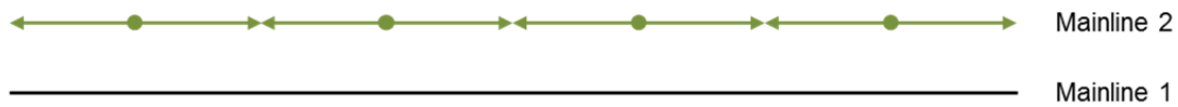
Figure 5.1: Alternating build-out strategy where four midpoints are chosen along the corridor, and second mainline track is built out in each direction
