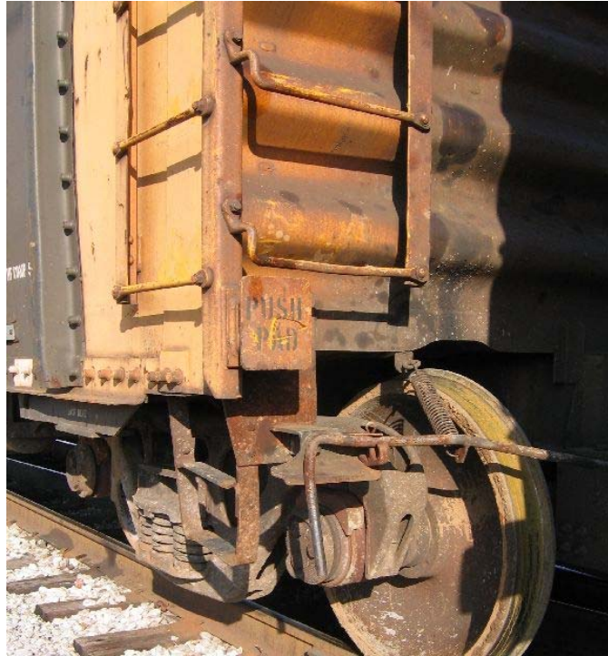
Figure 9.17 Sill step viewed from shallow angle to show sill step deformation
