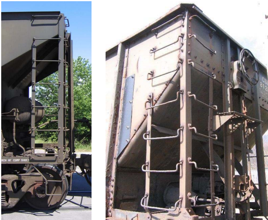
Figure 9.19 Images of the side ladder (left) as well as an image of both the side and end ladders (right) on open-top hopper cars
