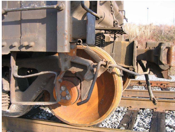
Figure 9.31 Example of an uncoupling lever
