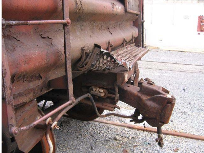
Figure 9.12 End platform on a boxcar showing significant deformation
