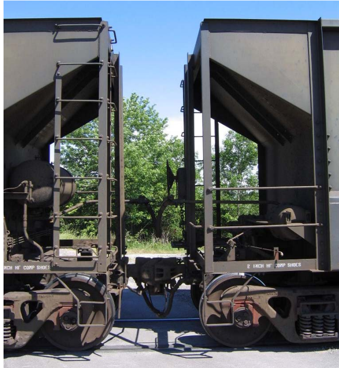
Figure 9.24 Side handholds on both the AL and BR corners of open-top hopper cars
