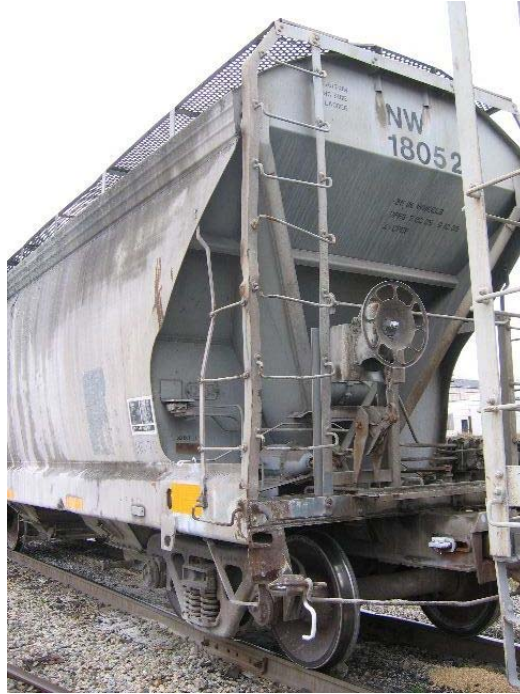
Figure 9.22 Deformations of side and end ladders on a covered hopper car
