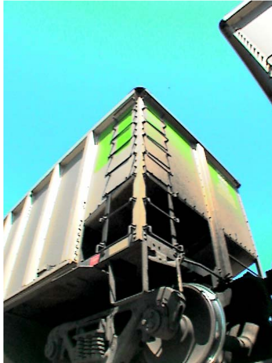
Figure 7.5 Upward angled side view of railcar representing the optimal angle for viewing ladder, handholds, and the brake wheel
