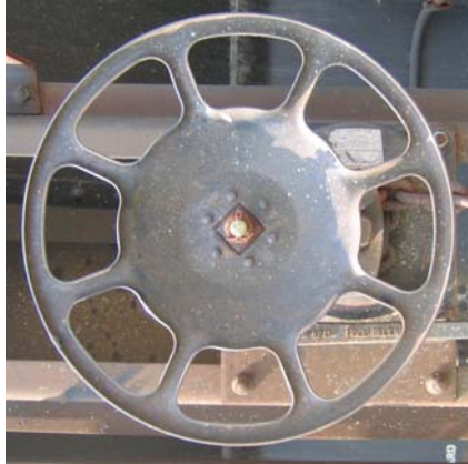
Figure 9.2 Profile view of a common brake wheel design
