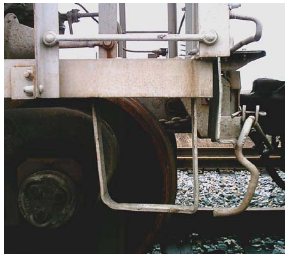
Figure 9.13 Sill step without additional rung
