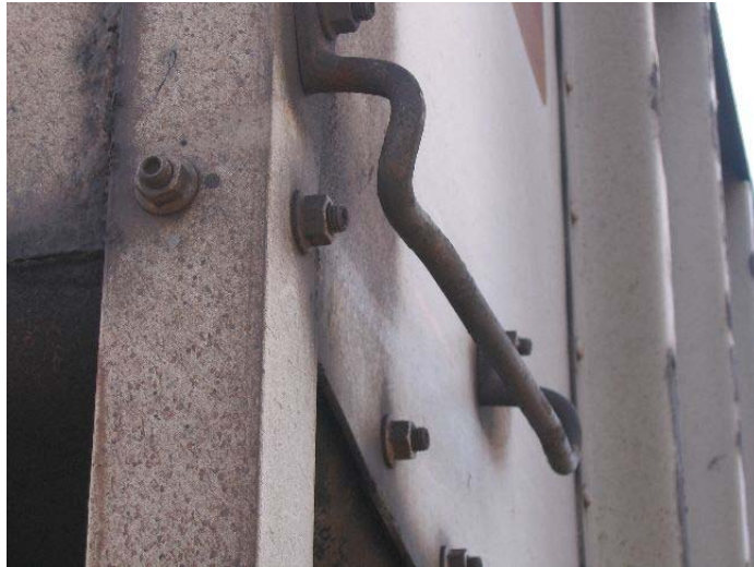
Figure 9.26 Side handhold on an open-top hopper car showing less than the required 2" clearance
