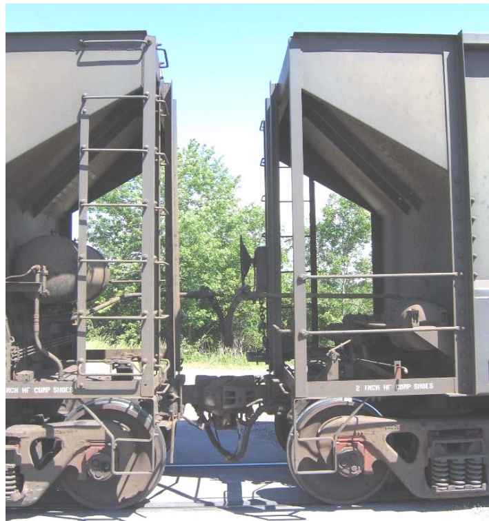
Figure 9.5 Brake wheel viewed from perpendicular to the track showing brake wheel clearance
