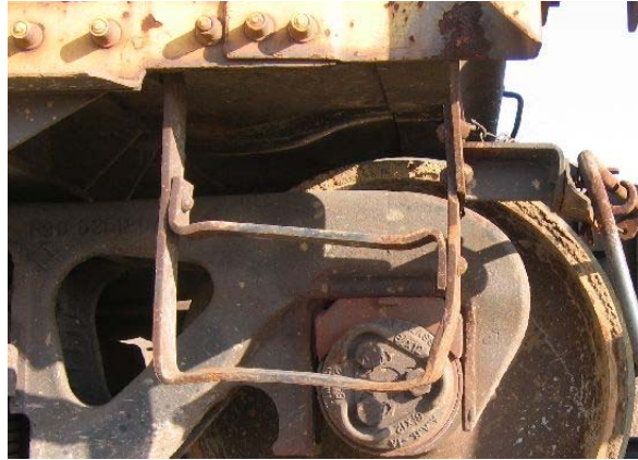
Figure 9.14 Sill step with additional rung
