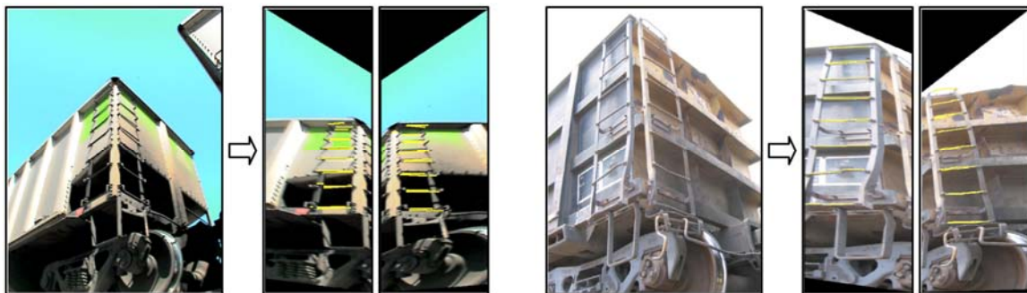
Figure 7.14 Additional examples of detected ladder rungs and handholds
