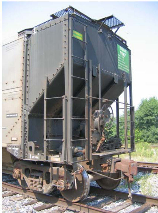
Figure 1.1 Picture of the end of a covered hopper car showing the safety appliances: sill step, side and end ladder, brake step, side and end handholds, and the brake wheel
