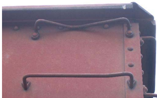
Figure 9.23 Deformations of the top side ladder rung on an open-top hopper car
