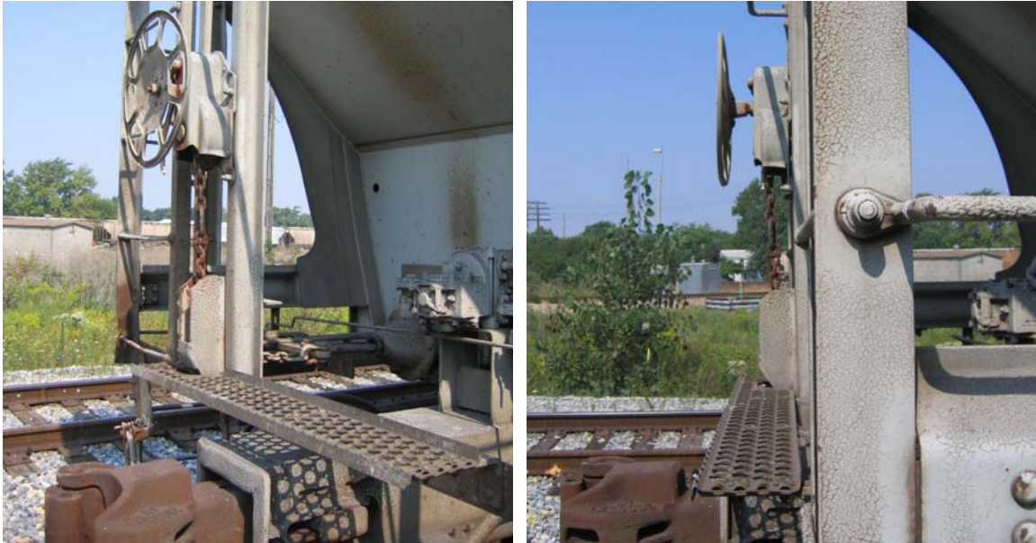
Figure 9.7 Example images of the brake step and brake wheel
