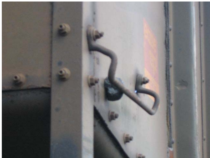
Figure 9.27 Side handholds clearance potentially affected by a piece of coal on an open-top hopper car
