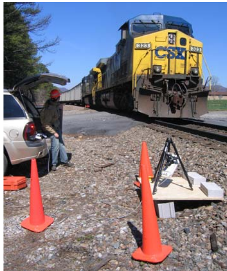
Figure 7.9 Temporary portable field setup for machine vision collection of safety appliance images
