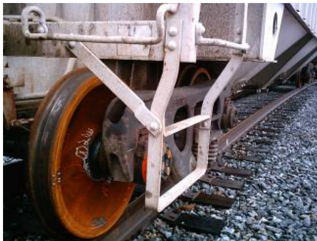
Figure 9.16 Sill step offset underneath the railcar
