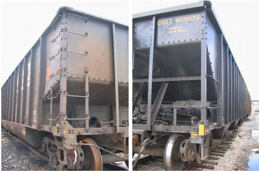
Figure 9.28 View of both the AR and BR corners of the railcar showing the horizontal end handholds on open-top coal cars
