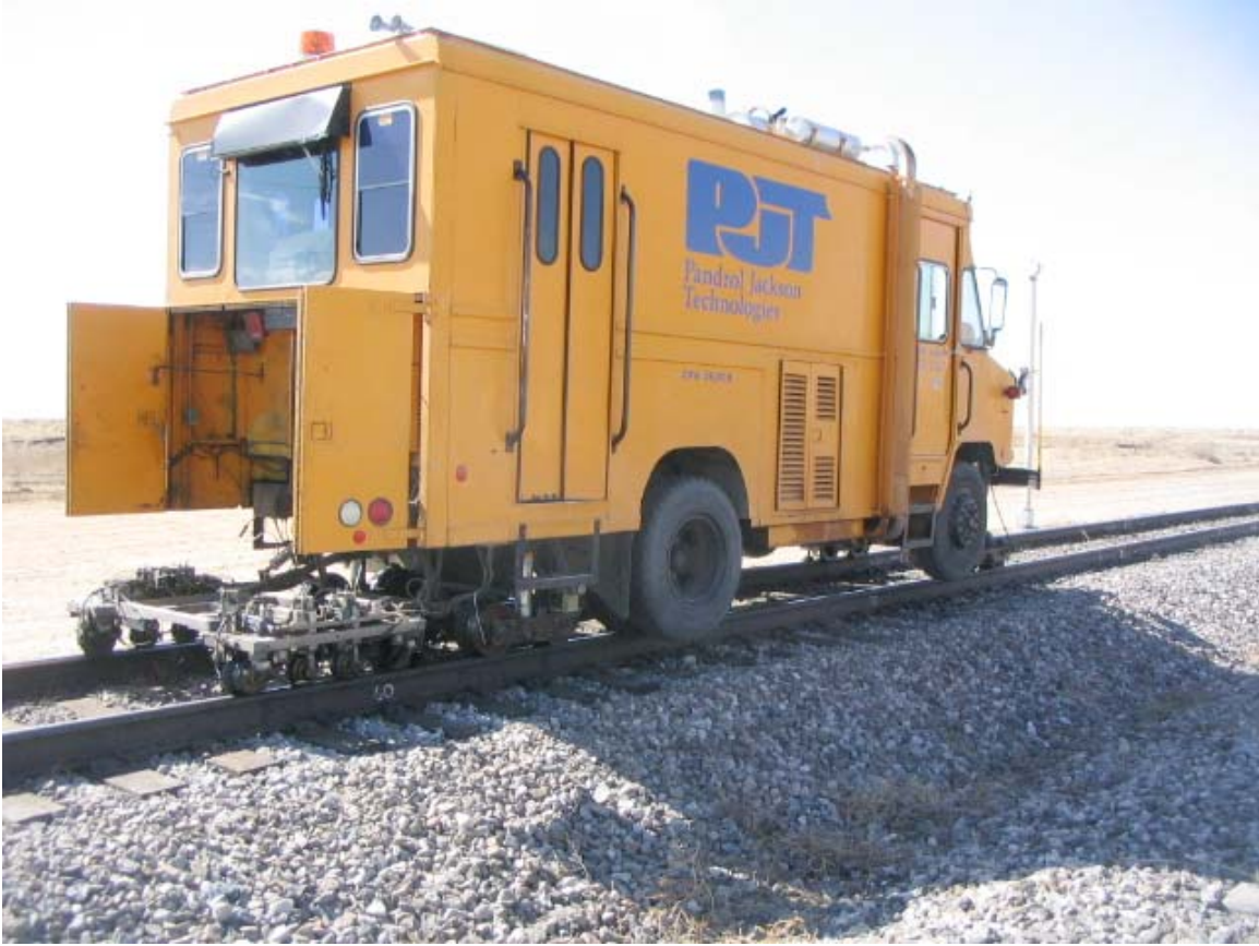
Figure 10.1 High-Rail Rail Flaw Detection Vehicle
