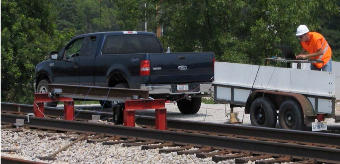
Figure 9.18 Data Acquisition Setup Next to CN Siding
