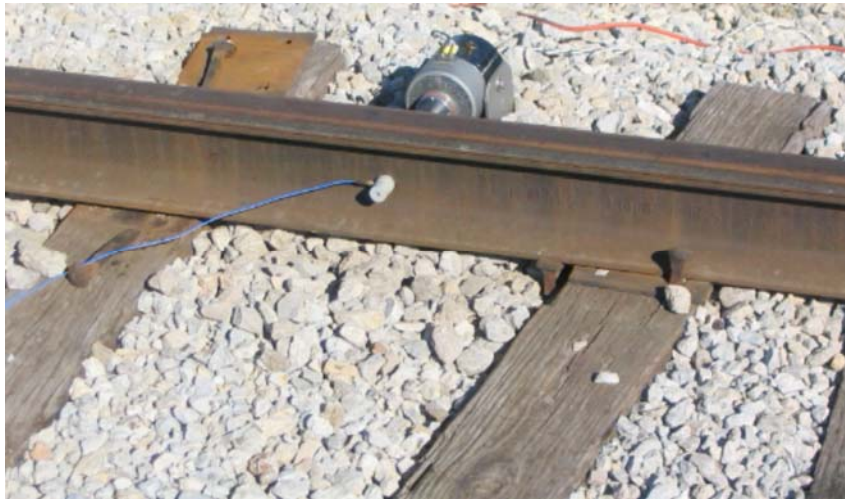
Figure 9.1 Accelerometer Monitoring Rail Vibrations
