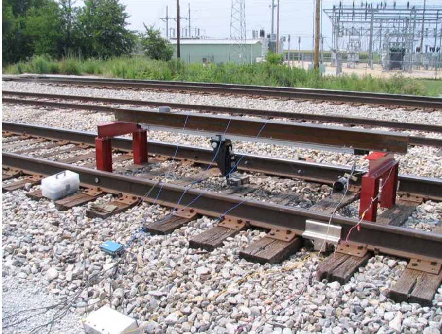
Figure 9.15 Field Test Setup on CN Siding
