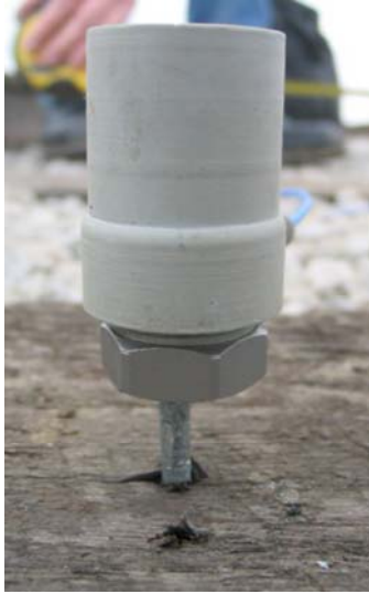
Figure 9.3 Magnetic-Based Accelerometer Attached to a Nail in Timber Ties
