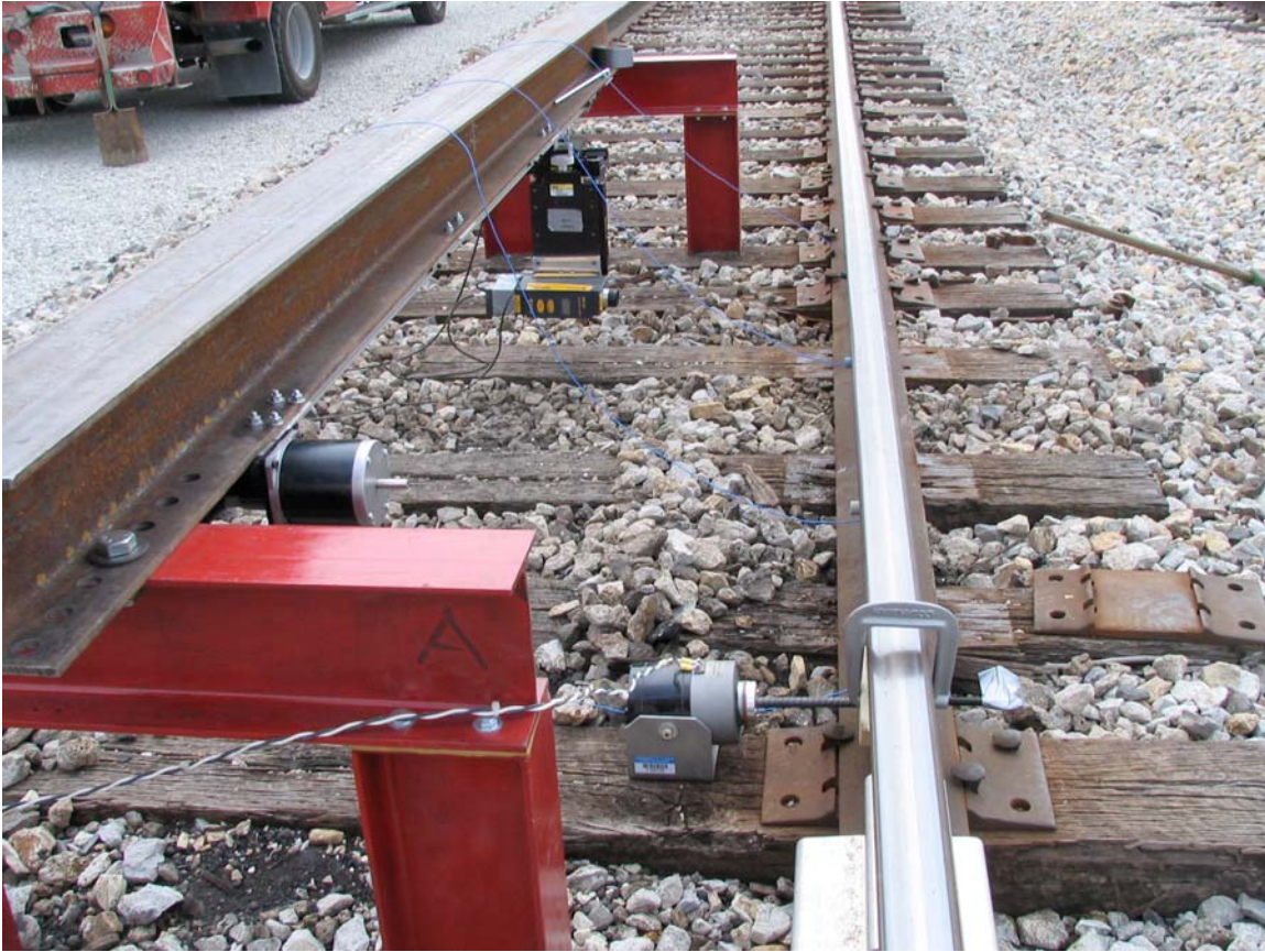
Figure 9.17 Accelerometer and Shaker Setup
