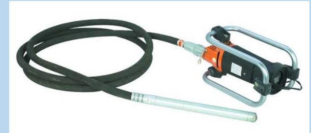
Plant C used handheld vibrator
