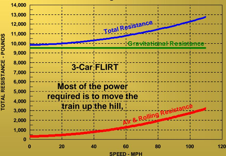
Train Power Requirements on 4 Percent Grade Horsepower Per Ton; Train Weight = 119 Tons
