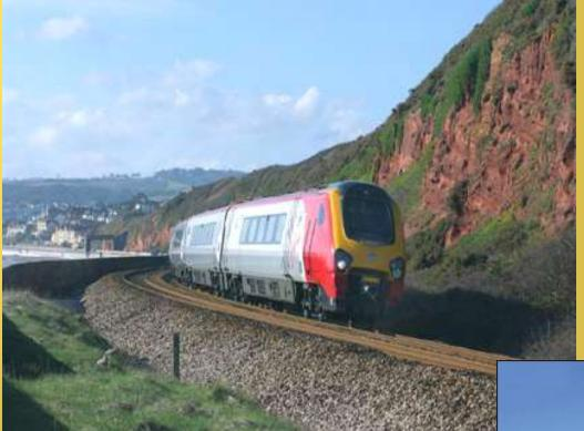
Bombardier Merdian family of DMU's – up to 200 km/h (120 mph), tilt and non-tilt versions.
