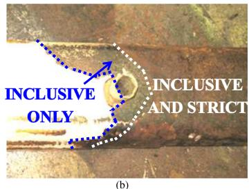
Figure 2: Disassembled IJ's. (a) Measuring the debonded region. (b) Inclusive versus Strict debonding.
