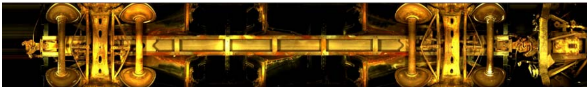
Figure 7.2 Panorama of Hopper Car Underframe Using Preliminary Image Acquisition Methods
