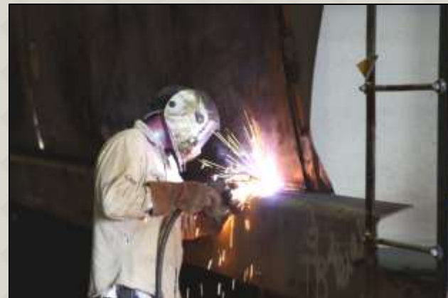
Employee at FreightCar America welding locomotive parts.
