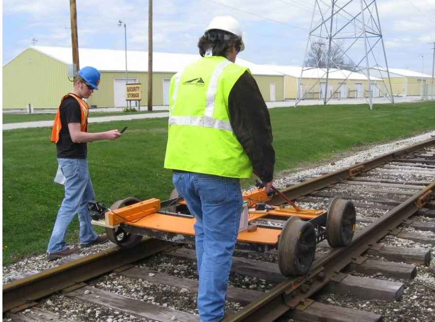
Figure 7.9: Recording Data While Timing Wheel Revolutions to Control Speed
