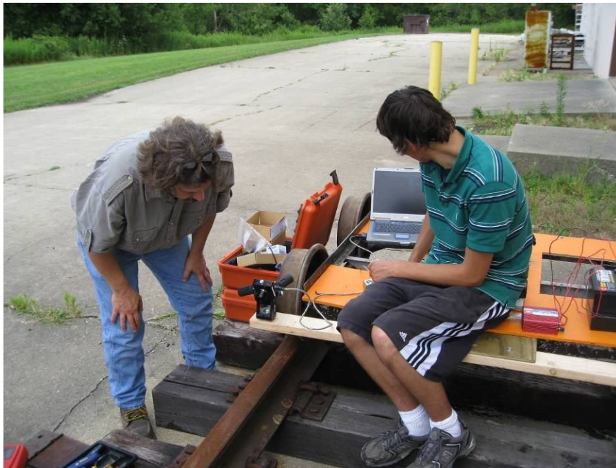
Figure 7.7: Adjustment of Camera Software Parameters on the VTC at the ATREL Track Panel
