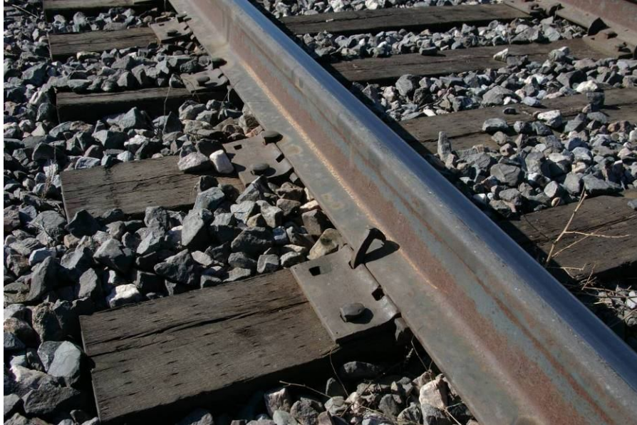
Figure 6.3: Image from Raised Spikes View Recorded at TTC's FAST
