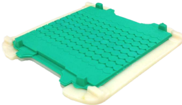
Figure 3.1 Rail pad assembly used for the laboratory and field tests
