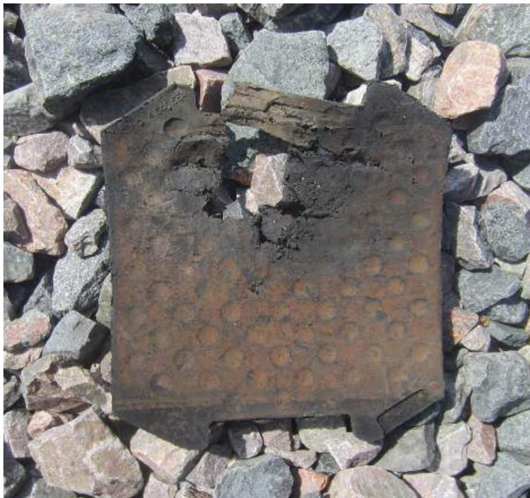
Figure 2.2 Tearing acting as a failure mode on rail pad assemblies
