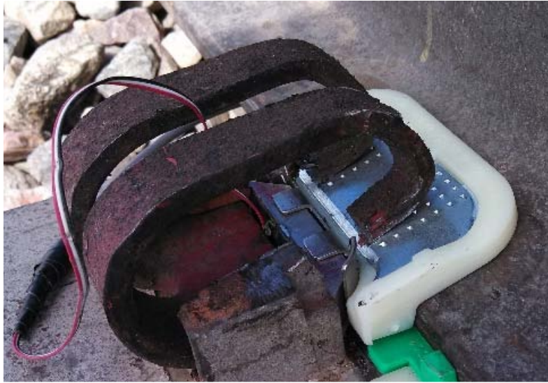
FIGURE 4. LLED Installed in Fastening System
