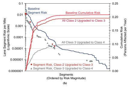
FIGURE 7 Effects of track infrastructure on risk: (a) effect of track class changes on risk as function of population density and (b) effect of infrastructure upgrade on risk reduction.
