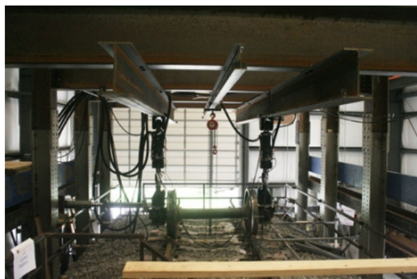
The Rail Transportation and Engineering Center features the state-of-the-art full-scale track loading system.
