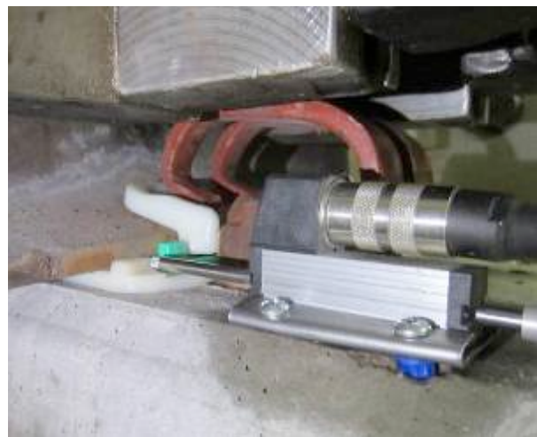
Figure 3 - Location of linear potentiometer
