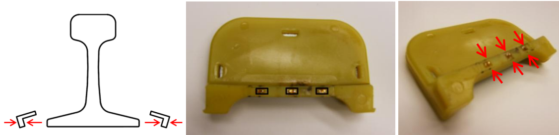
FIGURE 5: Insulator post compression; location of strain gauges; direction of strain (left to right).
