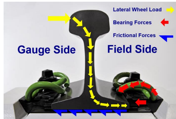
Figure 2. Hyperthetical lateral load path
