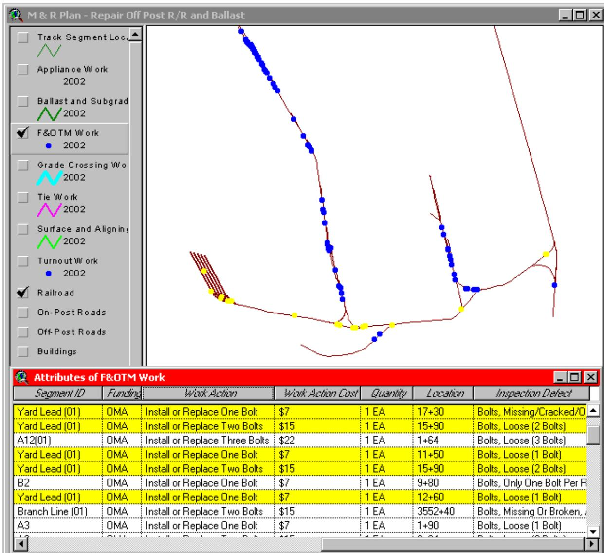
FIGURE 8 M&R Plan View illustrating individual work items on network highlighted for inclusion into plan.
