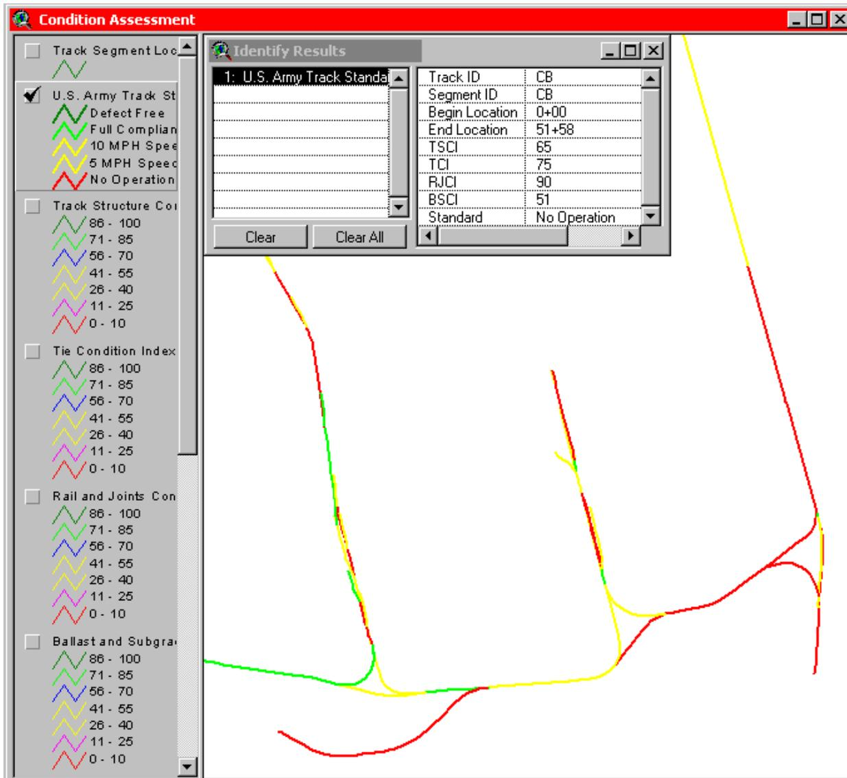
FIGURE 2 Condition Assessment View showing location of speed restrictions per the U.S. Army Track Standard.
