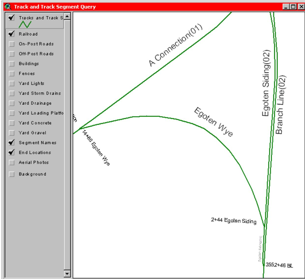
FIGURE 11 Track Segment Query View displaying overlay of segment names and end station locations.
