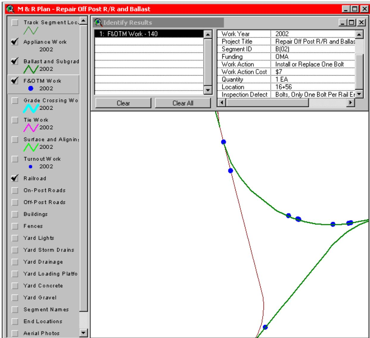
FIGURE 6 M&R Plan View displaying the location and other information for individual repair items.
