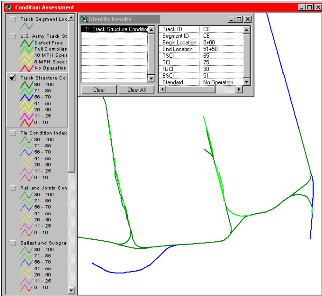
FIGURE 3 Condition Assessment View displaying TSCI ranges for network.
