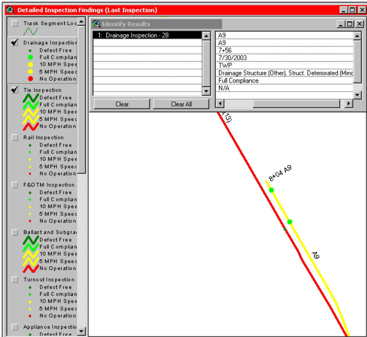
FIGURE 1 Detailed Inspection Findings View showing the interactive effect of drainage and tie defects.
