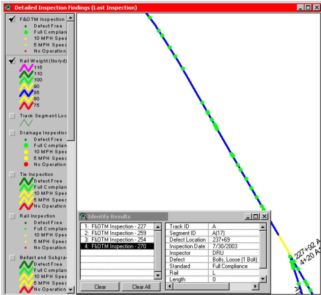
FIGURE 7 Detailed Inspection Findings View showing the high number of joint defects on light weight rail (85 lb).
