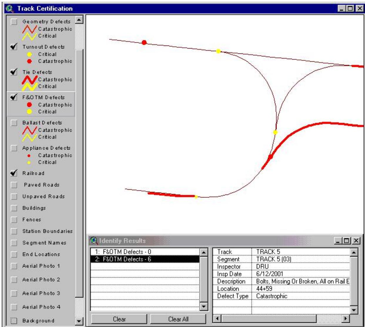
FIGURE 5 Track Certification View displaying critical and catastrophic defects causing certification restrictions.
