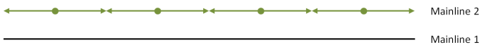
Figure 1: Alternating build-out strategy in which (not necessarily) four midpoints are chosen along the corridor, and second mainline track is built out in each direction
