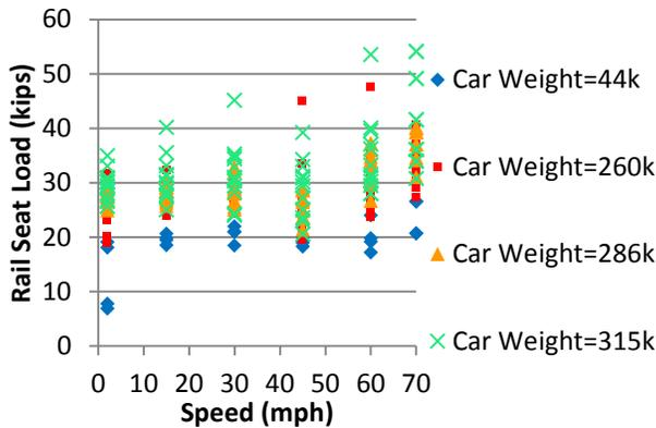
**FIGURE 11 RAIL SEAT LOADS AT RAIL SEAT U**
