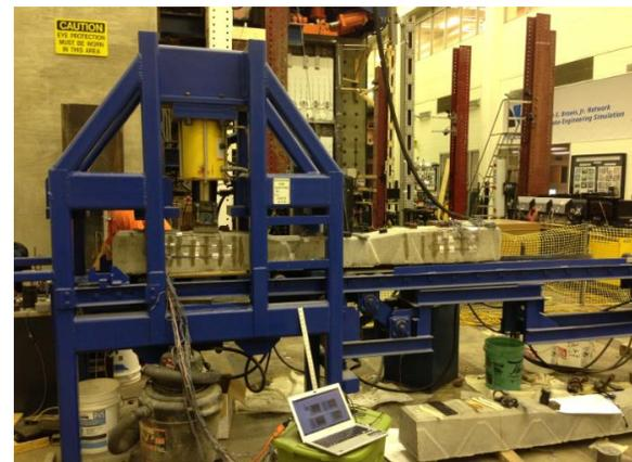
**FIGURE 1 STATIC TIE TESTER (STT)**
