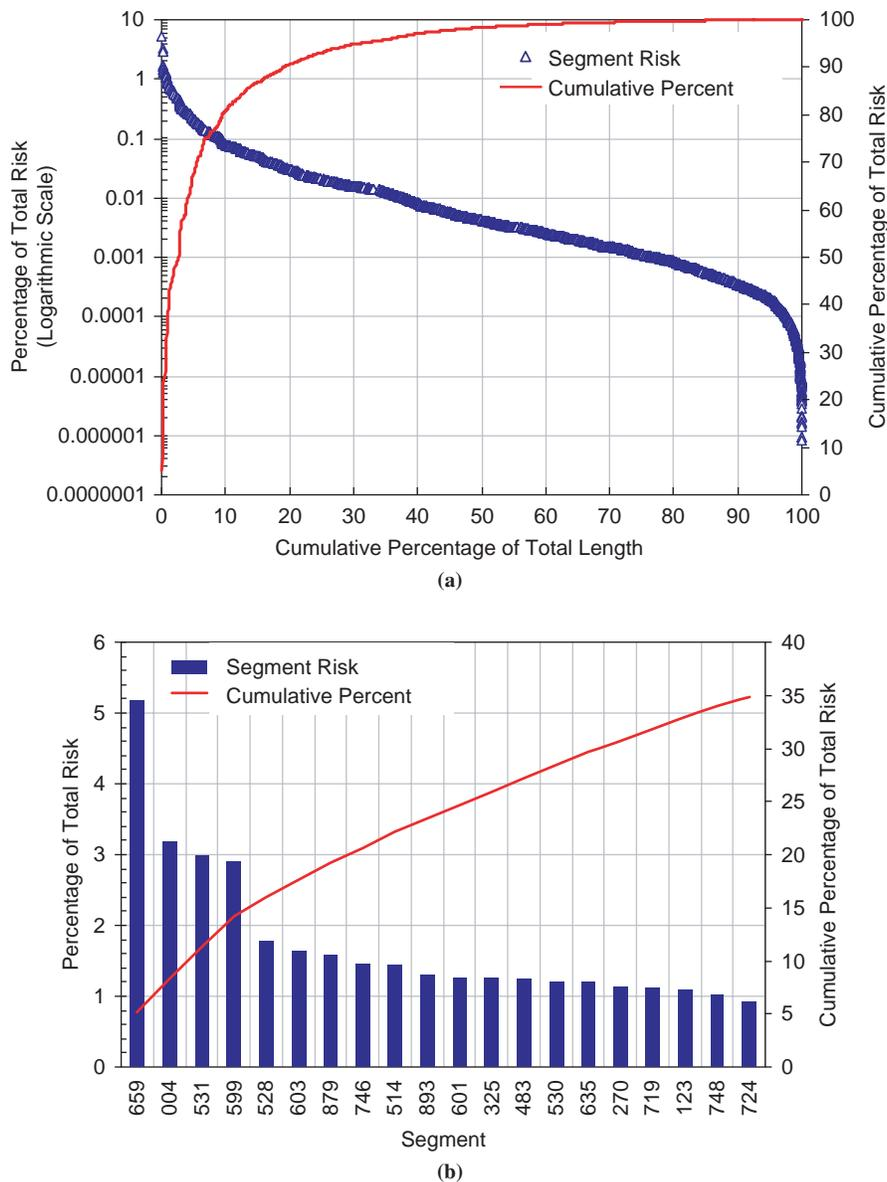
FIGURE 4 Graphical representation of combined lanes risk estimates: (a) all segments and (b) top 20 segments with the highest risk.
