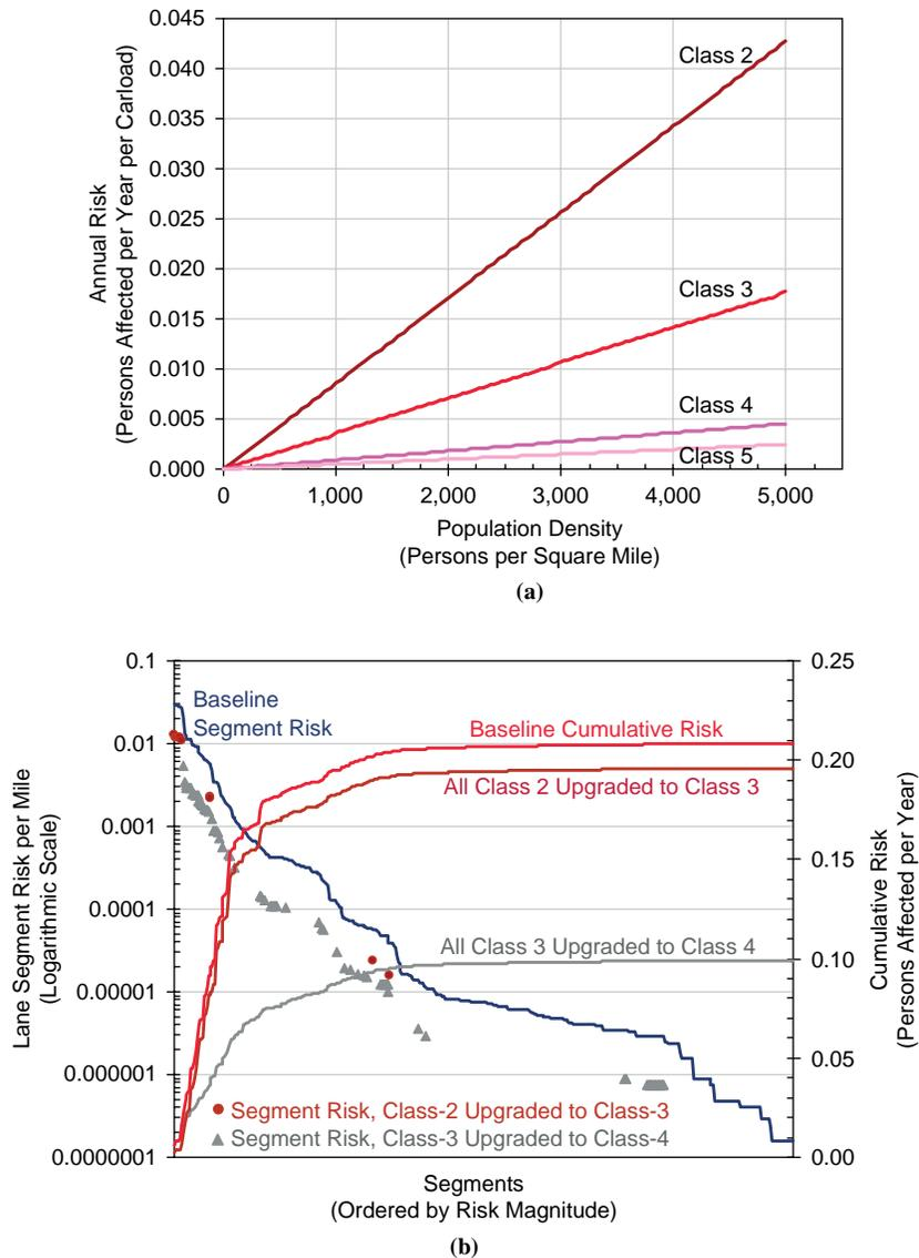
FIGURE 7 Effects of track infrastructure on risk: (a) effect of track class changes on risk as function of population density and (b) effect of infrastructure upgrade on risk reduction.
