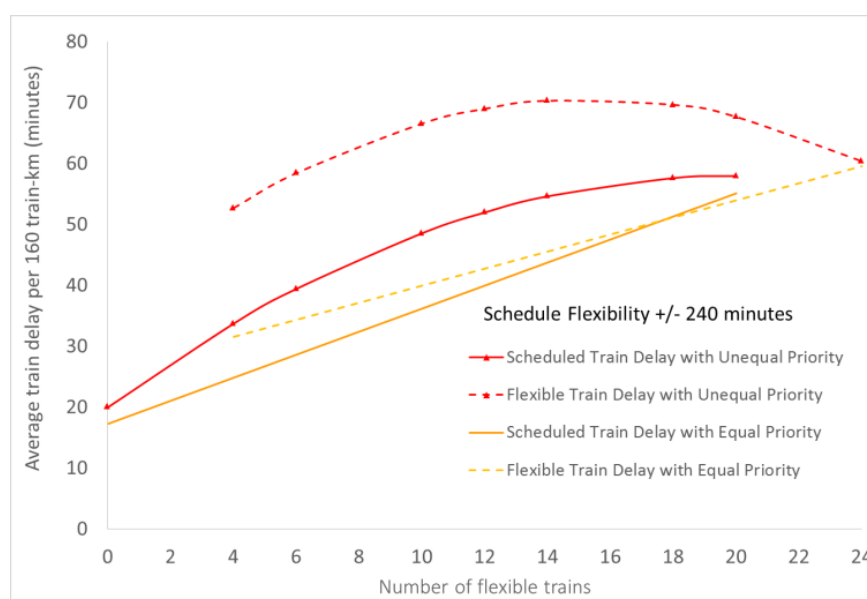
Figure 5: Scheduled and flexible average train delay with equal and unequal priorities for schedule flexibility of 240 minutes
