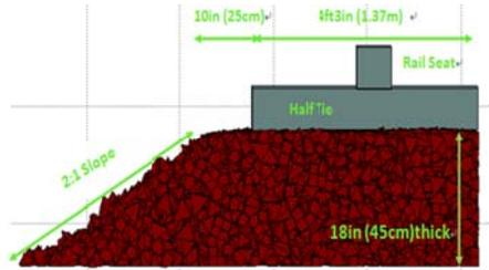
**Fig. 3 Front view of half-track model**
