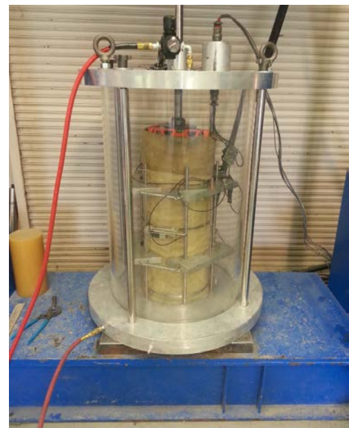
Figure 5. Photo of University of Illinois Ballast Triaxial Tester
