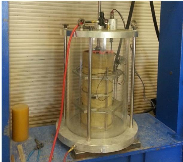
**FIG. 1. The University of Illinois ballast triaxial tester (TX-24)**
