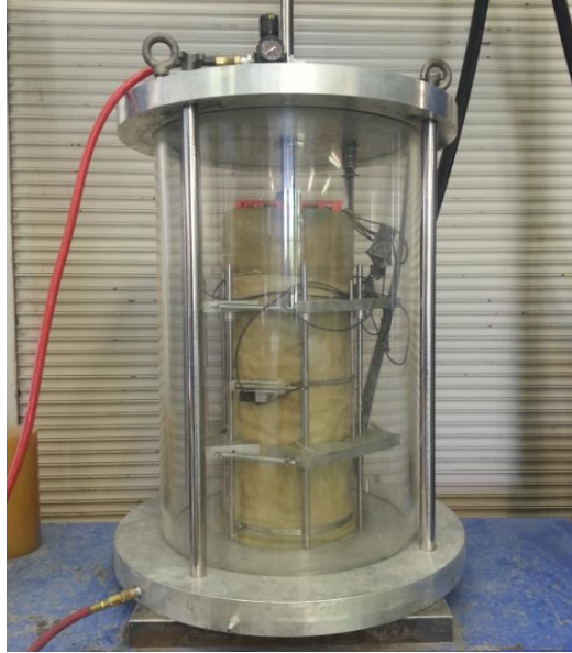
Figure 5. Photo of University of Illinois Ballast Triaxial Tester
