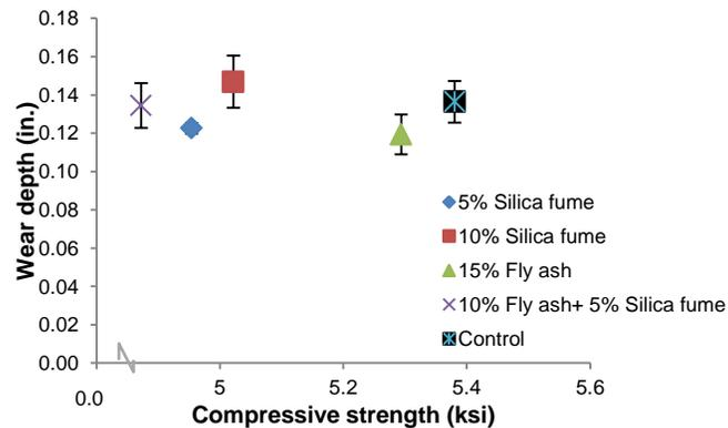
**FIGURE 3: WEAR DEPTH DEPENDENCE ON ADMIXTURE TYPE AND PROPORTION**
