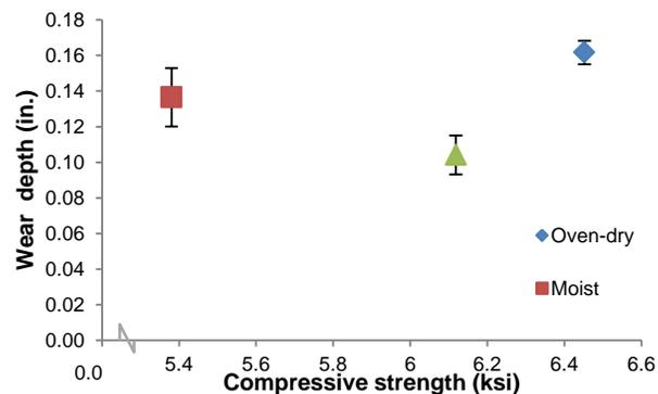
**FIGURE 4: WEAR DEPTH DEPENDENCE ON CURING CONDITION**
