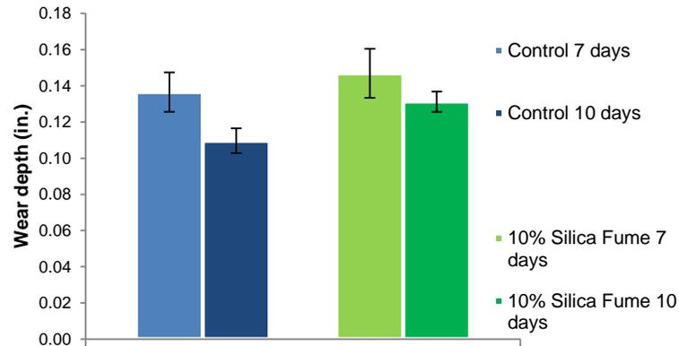
**FIGURE 5: WEAR DEPTH DEPENDENCE ON CURE TIME**
